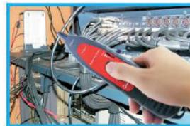
The sensitivity of the probe can be adjusted up or down with the slide control "SEN" . In case several cables are reacting to the tone probe, it helps by reducing the sensitivity of the probe downwards to only react to the right cable.
